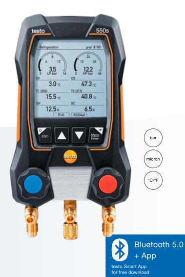
The testo 550s digital manifold with 2-way valve block enables you to carry out your measurements on refrigeration and air conditioning systems and heat pumps. The large display also helps you to evaluate the results in graphic form. Stored programs guide you through the measurement and enable the automatic determination of numerous important system parameters such as superheating/ subcooling, target superheat, cooling/heating capacity and many other areas besides.
